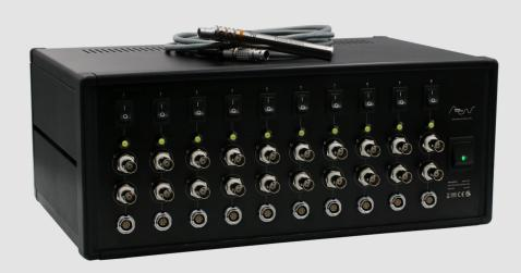
Weles Acoustics' Weles BOX X is a modular device designed to support up to 10 standard WA101  $^{1}/_{2}$ " PU Sound Probes. Each probe can be operated separately through a dedicated Weles BOX card equipped with its own individual power switch, probe input port and 2 analog BNC output channels - First channel for sound pressure, second for particle velocity.
